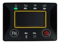
Figure 3-6: Internal UHF Radio LED
