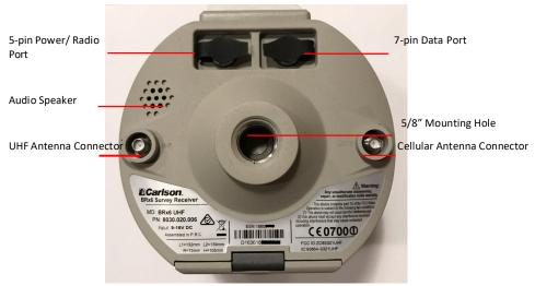
Figure 2-1: BRx6 ports and connectors
