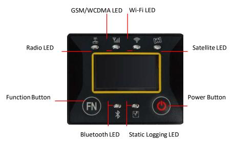
Figure 3-1: Control Panel and Display
